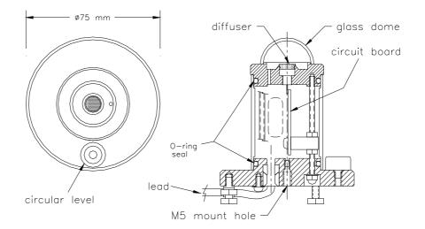
In-built signal amplifier to give a millivolt output for easy measurement. Chopper stabilised (for zero amplifier drift), with overvoltage & polarity reversal protection. SK01-D2 spectral response varies with wavelength so it is calibrated for solar spectral distribution and is not recommended for use in indirect or artifical lighting. Sealed to IP66, with internal desiccant (non-toxic silica-gel). User's Instructions and Calibration Certificate included.
