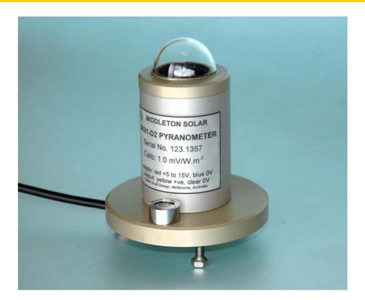
The SK01-D2 is a simple pyranometer for measuring total solar global radiation on a horizontal surface. The SKO1-DP2 version incorporates a special filter to limit its sensitivity to the **P**hotosynthetically **A**ctive **R**adiation region of the solar spectrum (400-700nm).
