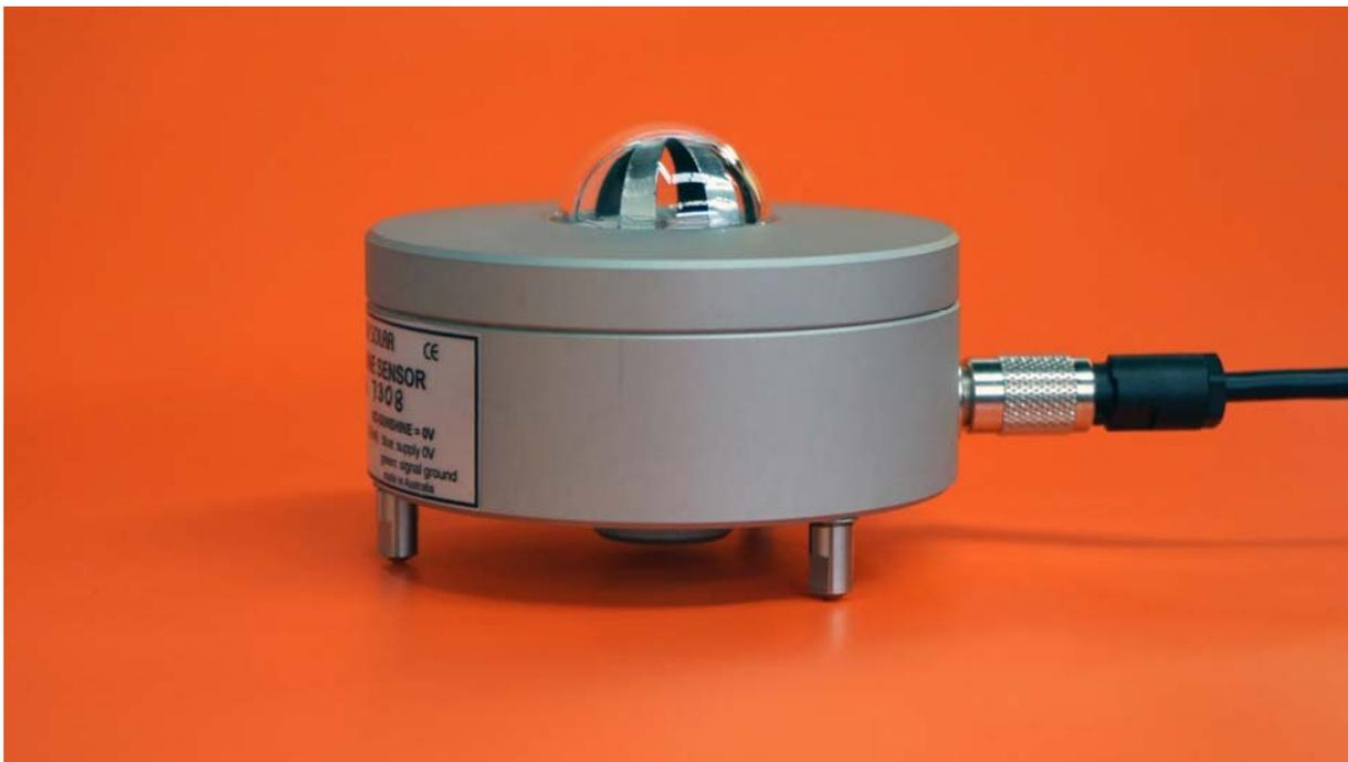
Four identical omni-directional sensors under a hemispherical shading canopy.
