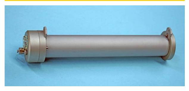
The Middleton Solar DN5-BF is a precision pyrheliometer for measuring the solar Direct Normal Irradiance (DNI) when aimed at the sun. It exceeds the International Organization for Standardization (ISO) specifications for a Fast Response Spectrally Flat Pyrheliometer of Class B. The DN5-BF has a compact thermopile sensor embedded in an integrating cavity, with the sensor not directly exposed to the sun to achieve very low zero off-set.
