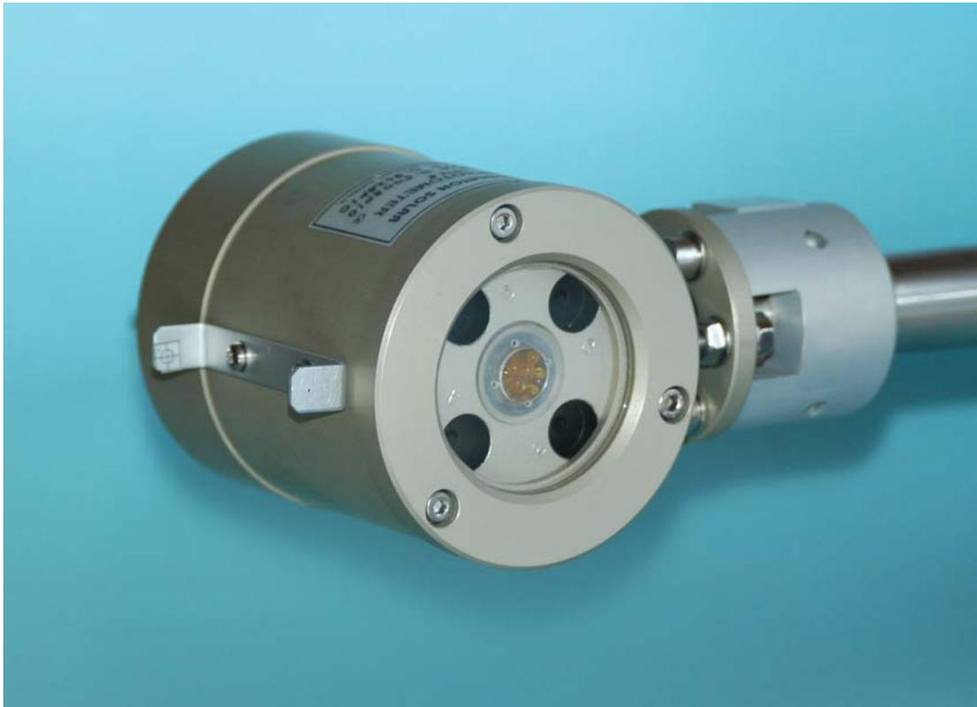
The Middleton Solar SP02 Sunphotometer is a simple low-cost instrument for the determination of the spectral optical depth of the atmosphere. It can be configured for total & aerosol optical depth measurement, column ozone measurement, and assessment of water vapour amounts. It consists of four precision spectro-pyrheliometers axially aligned in a sealed enclosure. The SP02-L version has a 35mm longer body to give a narrower field of view.
