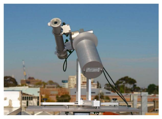
The Middleton Solar PST-01 Passive Solar Tracker is a basic equatorial mount designed to aim pyrheliometers and sunphotometers continuously at the sun throughout the day<sup>1</sup>.
