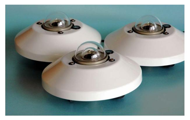
The Middleton EQ08-S is a precision pyranometer for the measurement of global solar irradiance on a plane surface. It exceeds the international accepted specifications for a high quality pyranometer. The EQ08-S incorporates a second generation precision thermoelectric sensor that has exceptionally low directional error without compromise to signal strength or response time. The EQ08-SE version has an in-built amplifier to give a millivolt output for easy signal measurement.
