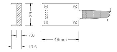
Temperature difference between the top and bottom faces generates a DC voltage output from the sensor thermopile.
