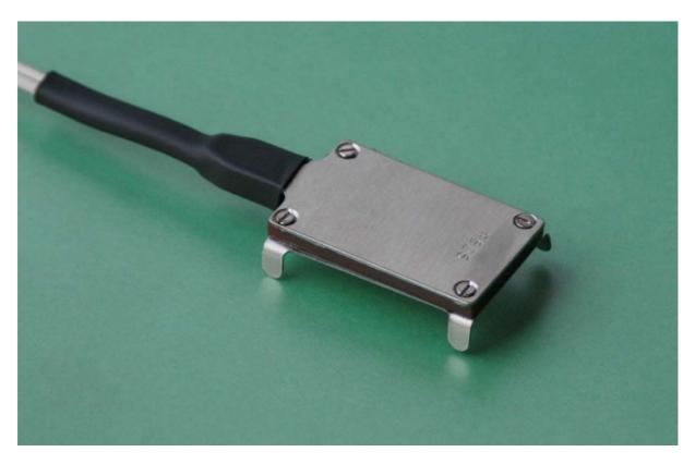
The Middleton CN3 Heat Flux Plate measures conductive heat transmission in the medium in which it is buried. It can be used for soil energy balance measurement and for determining heat transfer in walls, roads and bridges.
